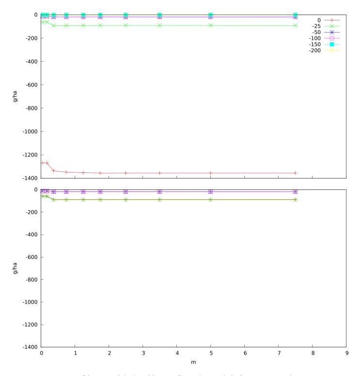
Figure B.31: Silstrup total (top) and biopore (bottom) vertical glyphosate transport between 2001-5-1 and 2002-3-1. The transport is shown on the y-axis (positive up) as a function of distance from drain shown on the x-axis. The graph labels are depths in centimeters above surface.
