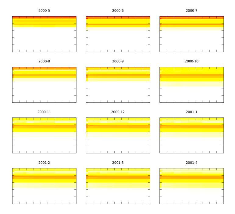
Figure B.23: Silstrup metamitron soil water concentration at the end of each month since first application of bromide. The y-axis denotes depth, the x-axis distance from drain. There are tick marks for every meter. The color scale is white<10 pg/l, yellow=1 ng/l, orange=0.1  $\mu$ g/l, red=10  $\mu$ g/l, and black>1 mg/l
