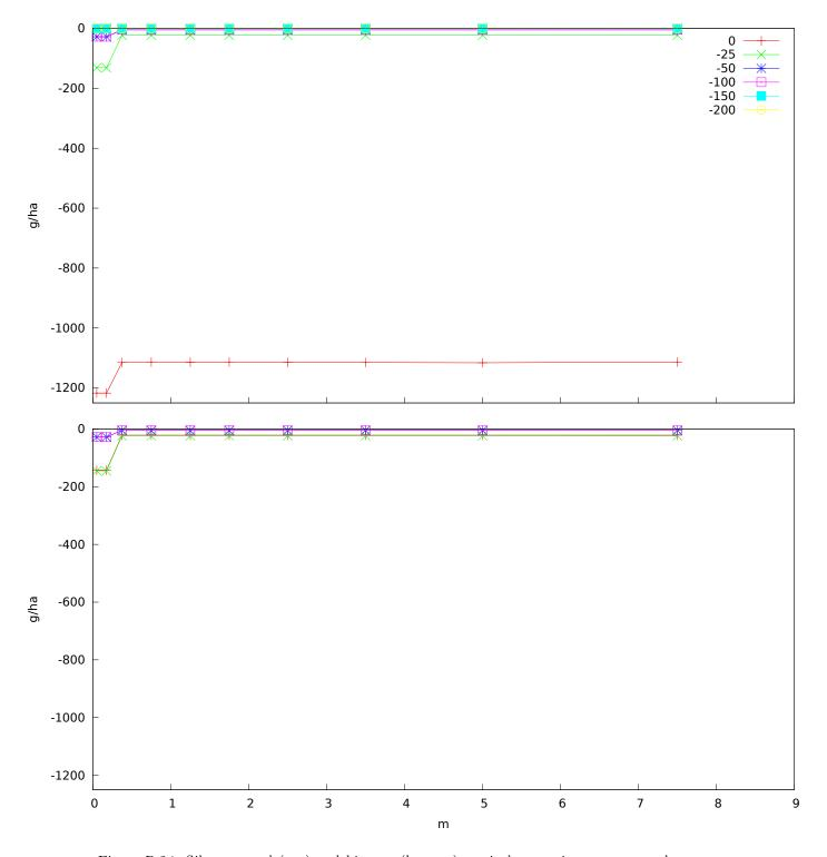
Figure B.24: Silstrup total (top) and biopore (bottom) vertical metamitron transport between 2000-5-1 and 2001-5-1. The transport is shown on the y-axis (positive up) as a function of distance from drain shown on the x-axis. The graph labels are depths in centimeters above surface.
