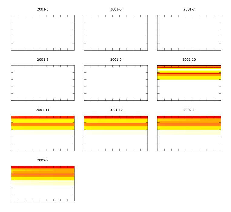
Figure B.25: Silstrup glyphosate soil content at the end of each month since one year after the first application of bromide. The y-axis denotes depth, the x-axis distance from drain. There are tick marks for every meter. The color scale is white<10 pg/l, yellow=1 ng/l, orange=0.1  $\mu$ g/l, red=10  $\mu$ g/l, and black>1 mg/l
