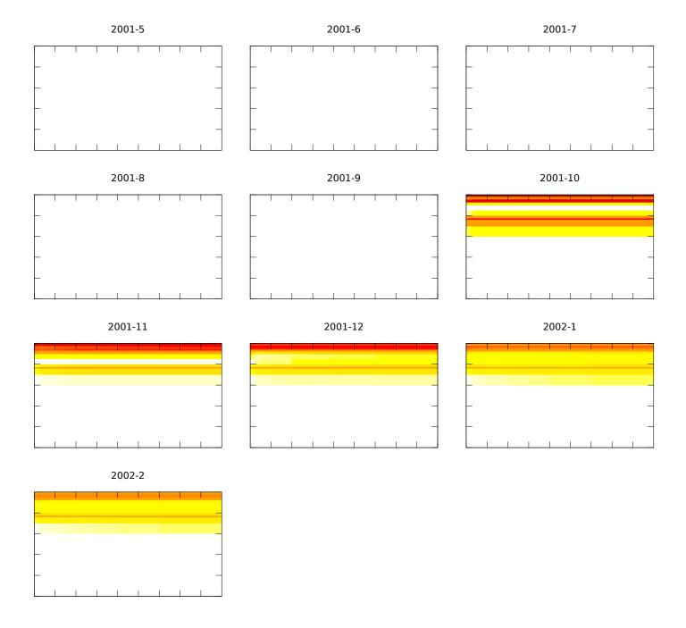
Figure B.26: Silstrup glyphosate soil water concentration at the end of each month since one year after first application of bromide. The y-axis denotes depth, the x-axis distance from drain. There are tick marks for every meter. The color scale is white<10 pg/l, yellow=1 ng/l, orange=0.1  $\mu$ g/l, red=10  $\mu$ g/l, and black>1 mg/l
