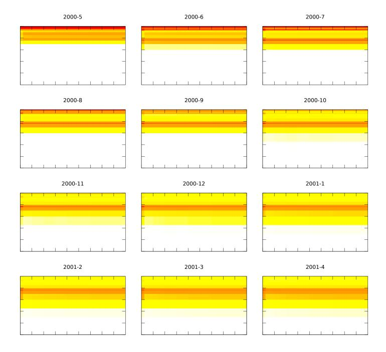
Figure B.22: Silstrup metamitron soil content at the end of each month since first application of bromide. The y-axis denotes depth, the x-axis distance from drain. There are tick marks for every meter. The color scale is white<10 pg/l, yellow=1 ng/l, orange=0.1  $\mu$ g/l, red=10  $\mu$ g/l, and black>1 mg/l
