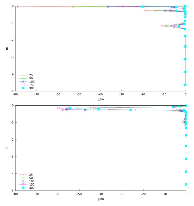
Figure B.30: Silstrup total horizontal glyphosate transport between 2001-5-1 and 2002-3-1 and Estrup total horizontal glyphosate transport between 2000-5-1 and 2001-5-1. The transport is shown on the x-axis (positive away from drain) as a function of depth shown on the y-axis. The graph labels are the distance from drain in centimeters.
